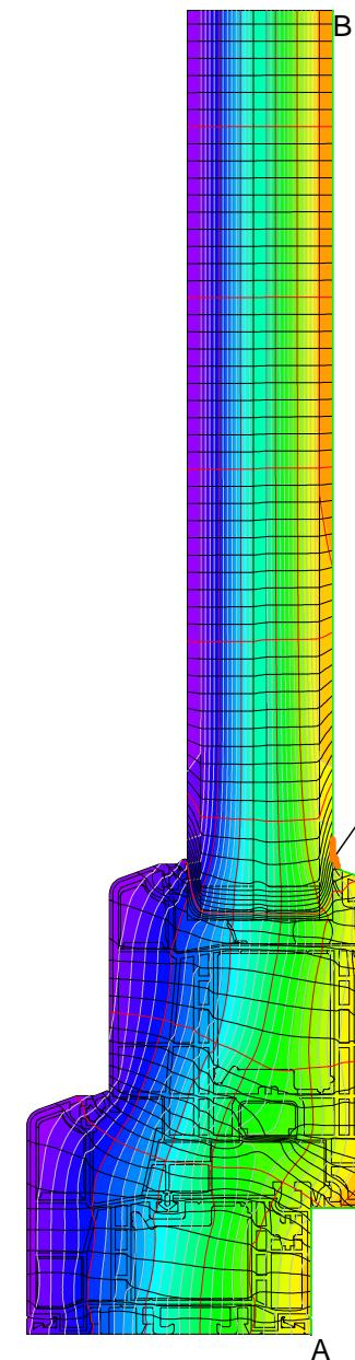
$$U_{f,A,B} = \frac{\frac{\Phi}{\Delta T} - U_p \cdot b_p}{b_f} = \frac{\frac{8,588}{30,000} - 0,701 \cdot 0,258}{0,142} = 0,743 \text{ W/(m}^2\text{·K)}$$
