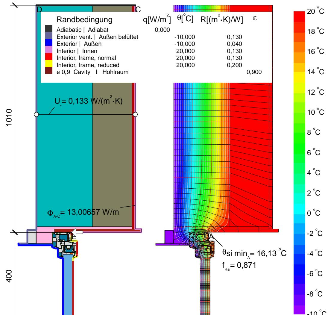
$$\psi_{A-E-C,*} = \frac{\Phi}{\Delta T} - U_1 \cdot b_1 - \frac{\Phi_2}{\Delta T} = \frac{13,436}{30,000} - 0,133 \cdot 1,010 - \frac{8,667}{30,000} = 0,024 \text{ W/(m}\cdot\text{K)}$$
