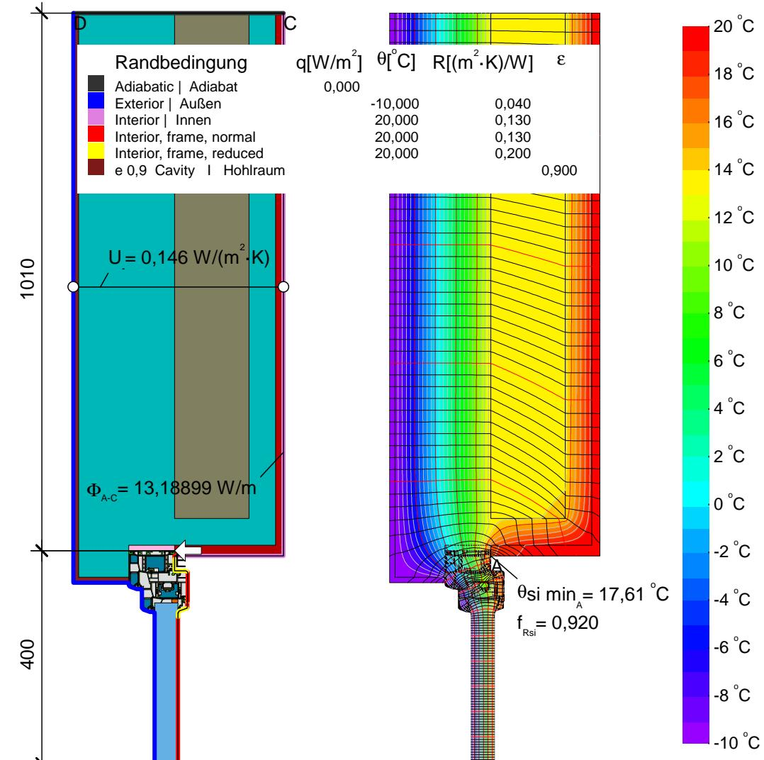
$$\psi_{A-E-C,*} = \frac{\Phi}{\Delta T} - U_1 \cdot b_1 - \frac{\Phi_2}{\Delta T} = \frac{13,538}{30,000} - 0,146 \cdot 1,010 - \frac{8,667}{30,000} = 0,015 \text{ W/(m·K)}$$
