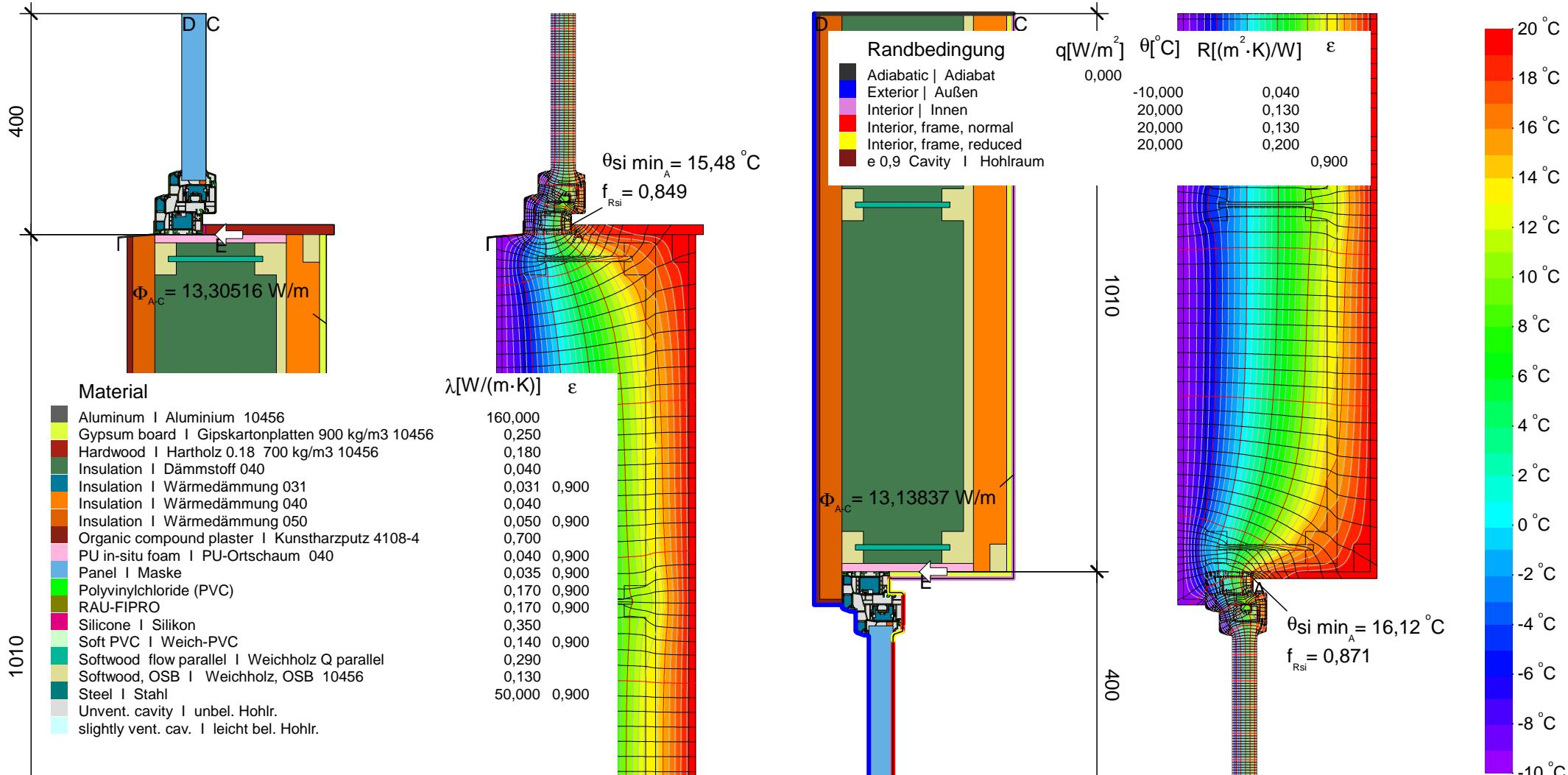
$$\psi_{A-E-C,*} = \frac{\Phi}{\Delta T} - U_1 \cdot b_1 - \frac{\Phi_2}{\Delta T} = \frac{13,305}{30,000} - 0,131 \cdot 1,010 - \frac{8,667}{30,000} = 0,022 \text{ W/(m}\cdot\text{K)}$$
