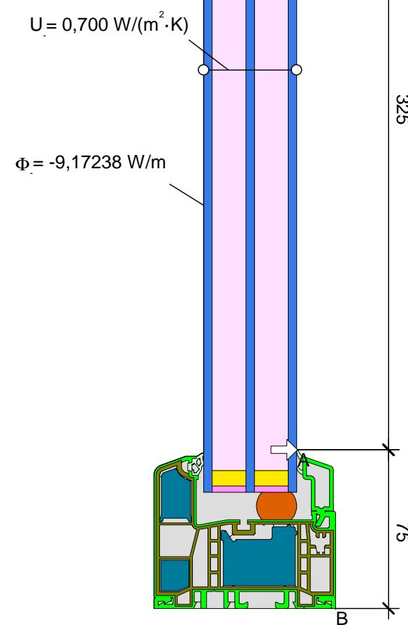
$$\psi_A = \frac{\Phi}{\Delta T} - U_g \cdot b_g - U_f \cdot b_f = \frac{9,172}{30,000} - 0,700 \cdot 0,325 - 0,697 \cdot 0,075 = 0,026 \text{ W}/(\text{m} \cdot \text{K})$$
