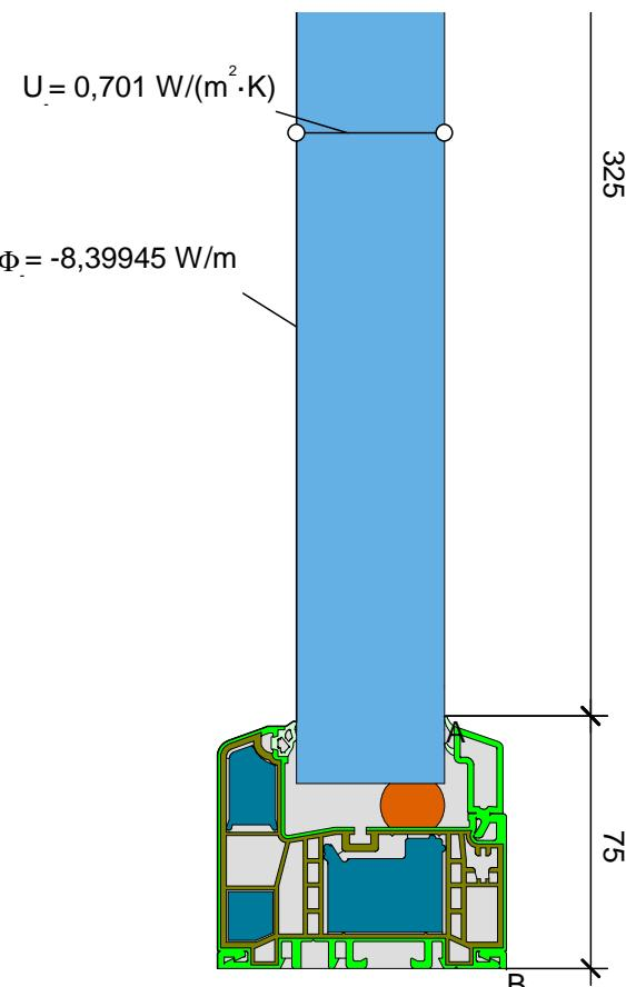
$$U_{f,A,B} = \frac{\frac{\Phi}{\Delta T} - U_p \cdot b_p}{b_f} = \frac{\frac{8,399}{30,000} - 0,701 \cdot 0,325}{0,075} = 0,697 \text{ W}/(\text{m}^2 \cdot \text{K})$$
