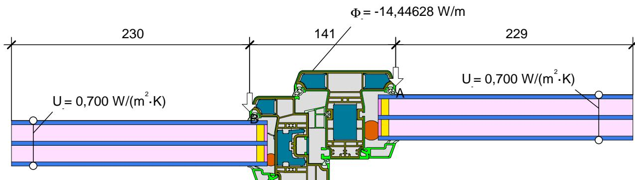
$$\Psi_{A,B} = \frac{\frac{\Phi}{\Delta T} - U_{g1} \cdot b_{g1} - U_f \cdot b_f - U_{g2} \cdot b_{g2}}{2} = \frac{\frac{14,446}{30,000}}{2} - \frac{0,700 \cdot 0,229 - 0,763 \cdot 0,141 - 0,700 \cdot 0,230}{2} = 0,026 \text{ W}/(\text{m} \cdot \text{K})$$
