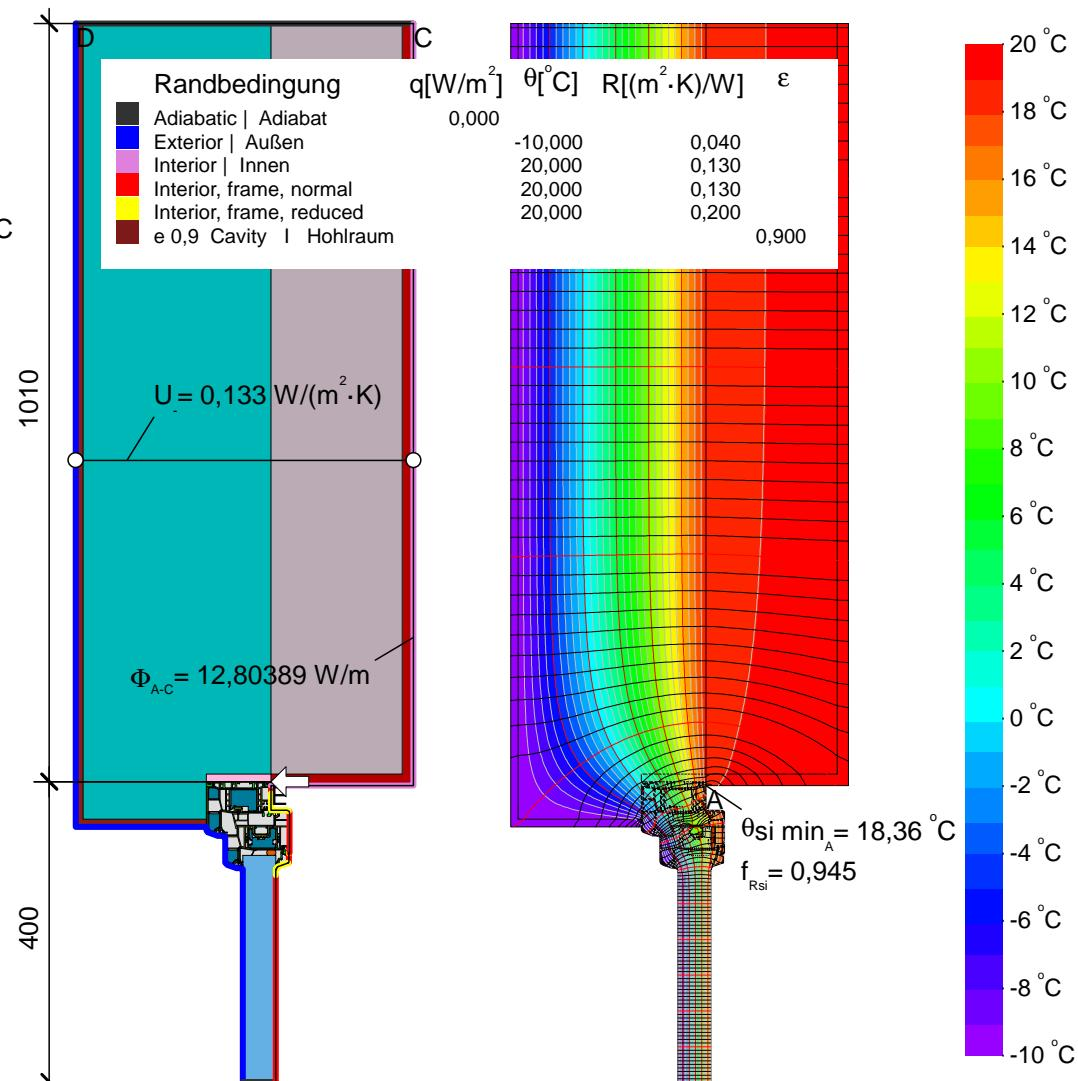
$$\psi_{A-E-C,*} = \frac{\Phi}{\Delta T} - U_1 \cdot b_1 - \frac{\Phi_2}{\Delta T} = \frac{13,288}{30,000} - 0,133 \cdot 1,010 - \frac{8,667}{30,000} = 0,020 \text{ W}/(\text{m} \cdot \text{K})$$
